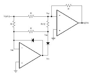
c) Make the input voltage an 8 Vpp sinusoid, at 200 Hz. Carefully measure and record voltages at all nodes in the circuit, using the notation for voltages shown in the schematic.
